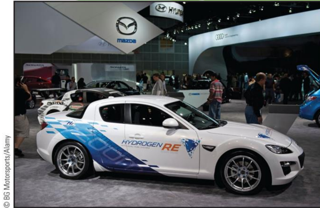
Figure 20.7: Mazda RX-8 RE, powered by a two-fuel internal combustion engine that runs on gasoline or hydrogen (CHG).
