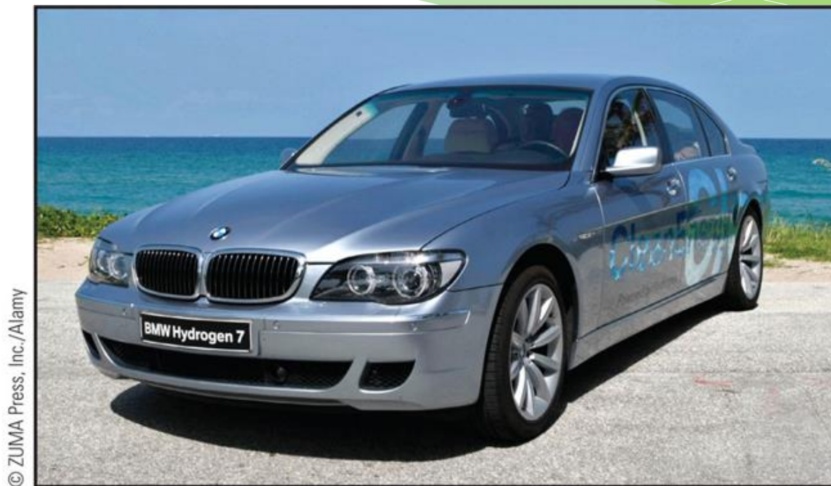
Figure 20.6: BMW Hydrogen 7 powered by a two-fuel internal combustion engine that runs on gasoline or hydrogen ( \text{LH}_2 ).
